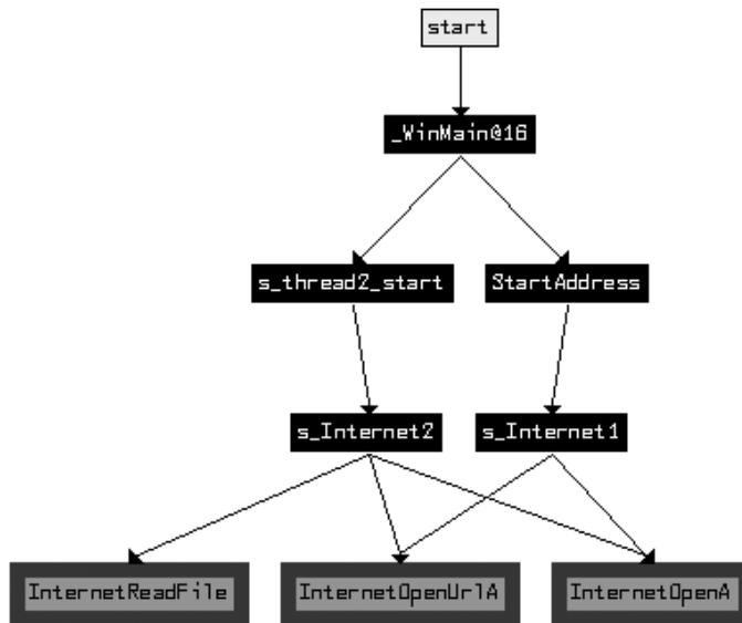
Figure 14-31: Function graph for functions connected with Internet functions
