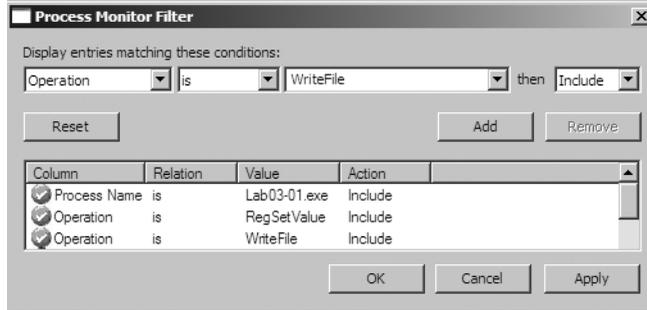
Figure 3-3L: Process Monitor Filter dialog showing filters set on Process Name and Operation
