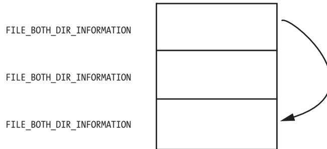
Figure 10-2L: A series of `FILE_BOTH_DIR_INFORMATION` structures being modified so that the middle structure is hidden
