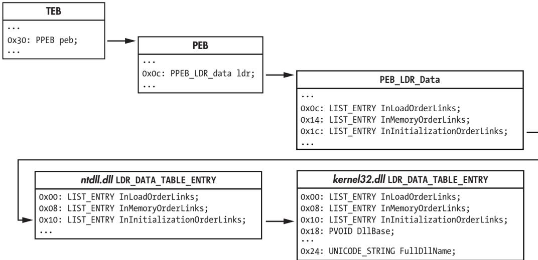
Figure 19-1: Structure traversal to find *kernel32.dll* *DllBase*
