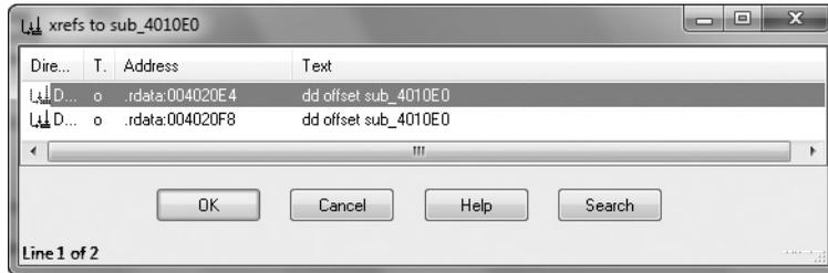
Figure 20-3: Cross-references for a virtual function
