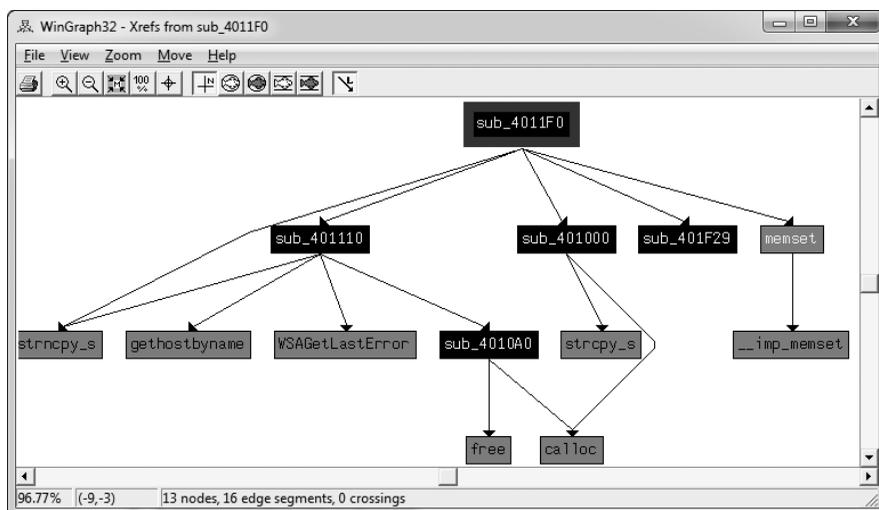
Figure 5-9: Cross-reference graph of a single function (`sub_4011F0`)
