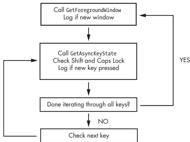
Figure 11-3: Loop structure of `GetAsyncKeyState` and `GetForegroundWindow` keylogger
