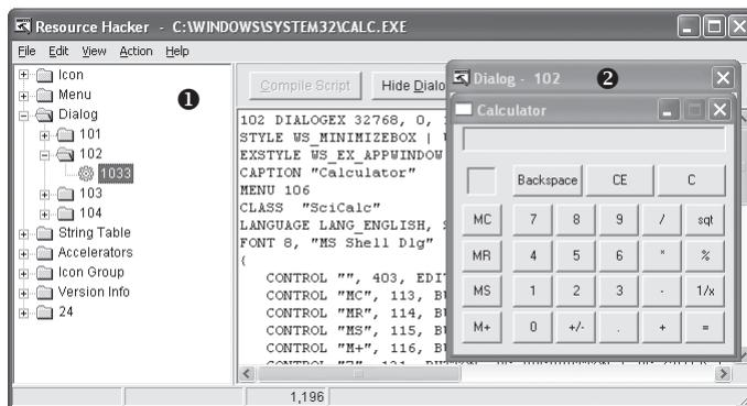
**Figure 1-9:** The Resource Hacker tool display for *calc.exe*
