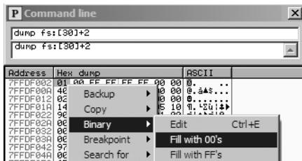
Figure 16-2L: Using the command line to dump the BeingDebugged flag and then setting it to 0
