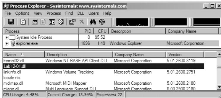
Figure 12-1L: Process Explorer view showing injected DLL
