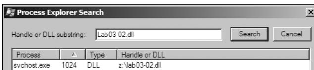
Figure 3-6L: Searching for a DLL in Process Explorer
