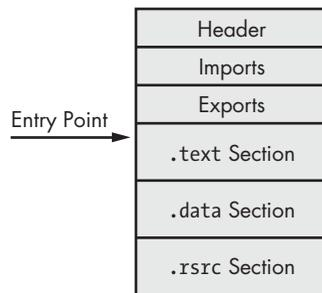
Figure 18-1: The original executable, prior to packing
