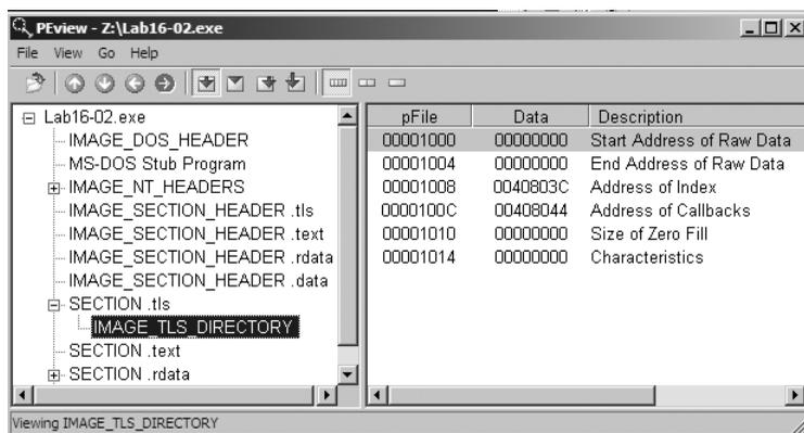
Figure 16-4L: PEView displaying a TLS section for Lab 16-2
