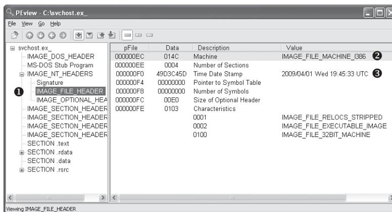
Figure 1-7: Viewing the `IMAGE_FILE_HEADER` in the PEView program
