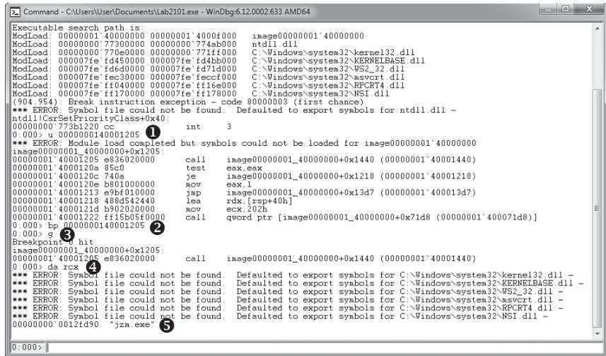
Figure 21-1L: Using WinDbg to see the string that is being compared in Lab 21-1
