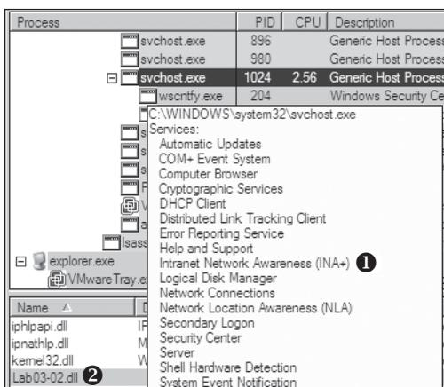
Figure 3-7L: Examining service malware in Process Explorer
