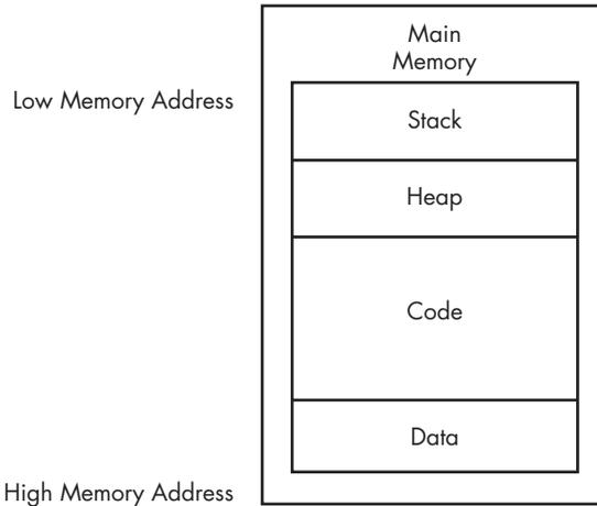
Figure 4-3: Basic memory layout for a program
