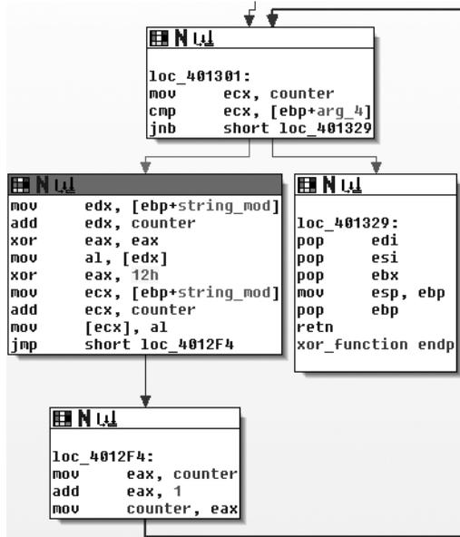
Figure 13-3: Graphical view of single-byte XOR loop
