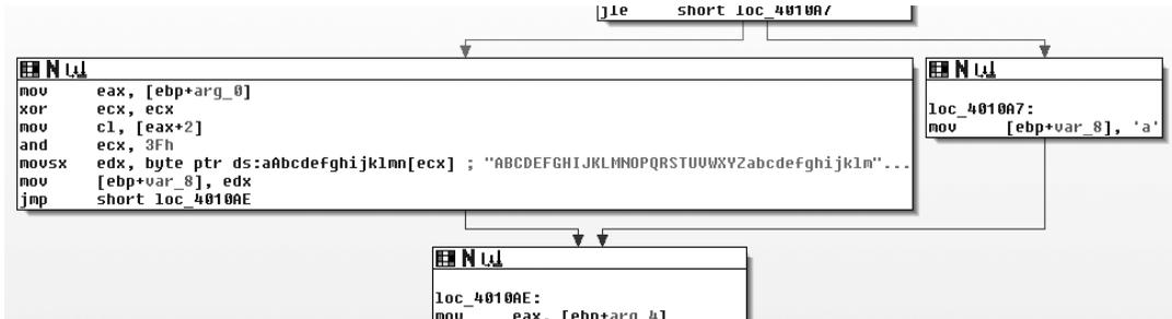
Figure 14-2L: Base64 encoding function (0x401000) with alternative padding
