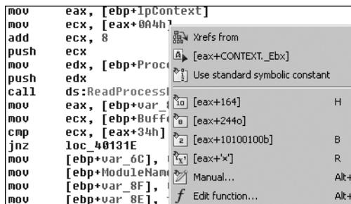
Figure 12-2L: IDA Pro structure offset resolution
