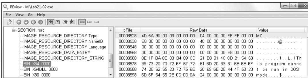
Figure 21-2L: PView showing three different resource sections
