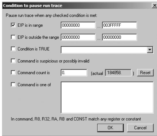
Figure 9-11: Conditional tracing
