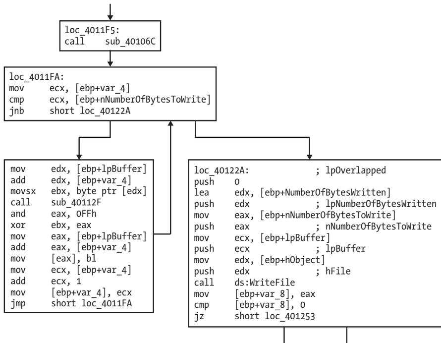
Figure 13-14: Function graph showing an encrypted write
