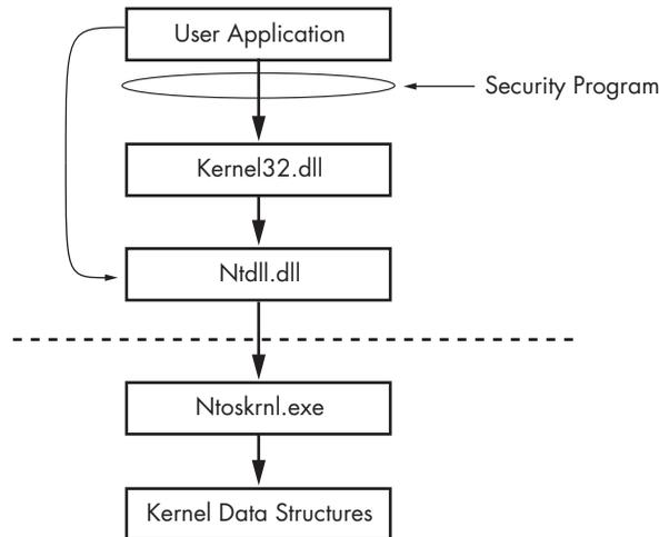
Figure 7-4: Using the Native API to avoid detection
