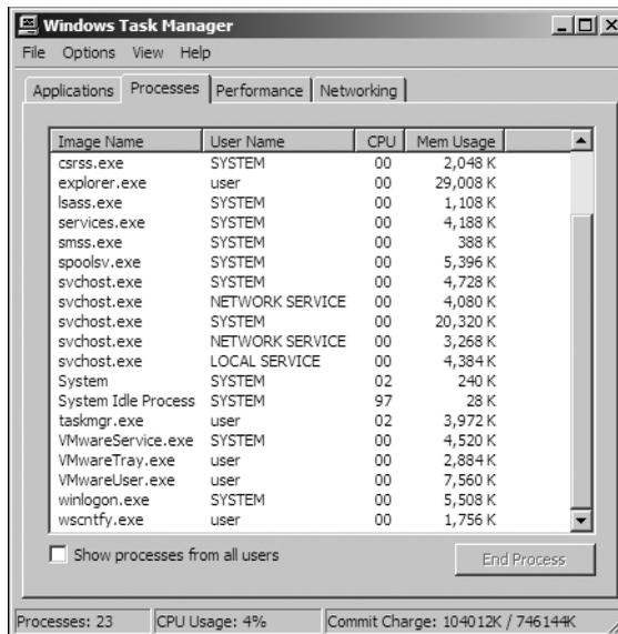
Figure 17-1: Process listing on a VMware image with VMware Tools running
