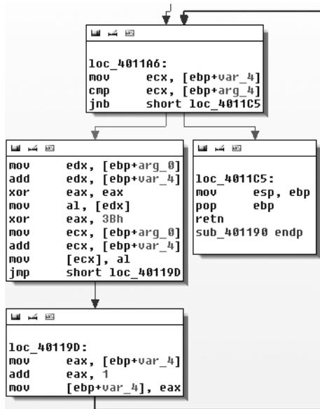
Figure 13-1L: Single-byte XOR loop with 0x3B in sub\_401190
