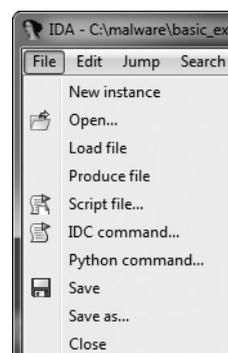
Figure 5-12: Options for loading IDC and Python Scripts
