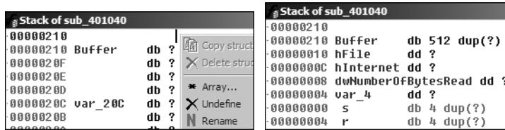
Figure 6-2L: Creating an array and fixing the stack
