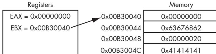
Figure 4-5: EBX register used to access memory
